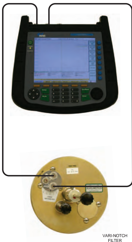
Figure 4: Checking the rejection notch.
